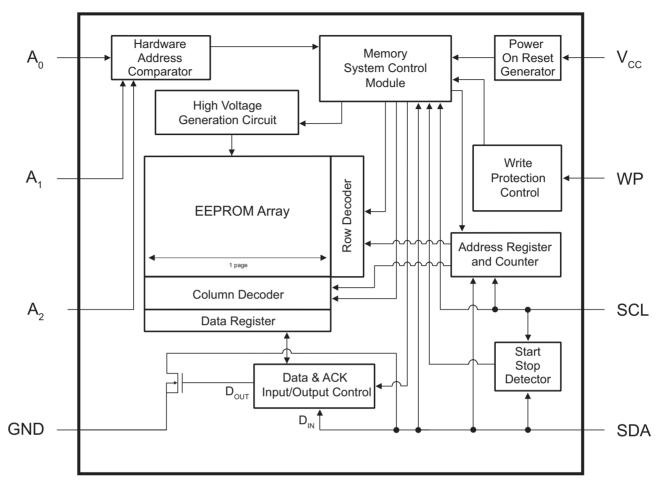
Figure 2-1. Block Diagram
