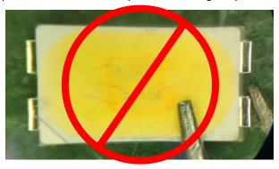
(2) In general, LEDs should only be handled from the side. By the way, this also applies to LEDs without a silicone sealant, since the surface can also become scratched.
