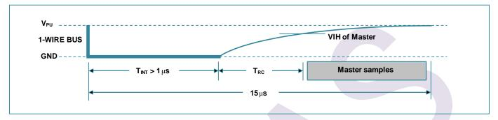
Figure 16. Recommended Master Read 1 Timing
