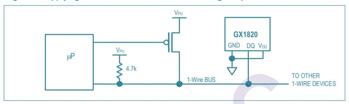
Figure 5. Powering the GX1820 with an External Supply
