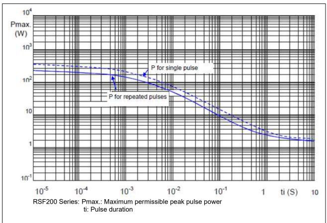
**Metal Oxide Film Resistors**
