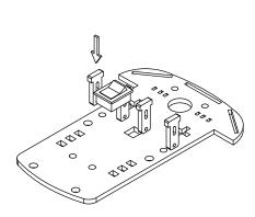
Setpl:Insert the fastener into the chassis after tearing off the yellow protection wrap of the chassis, the fastener and the code wheel.
