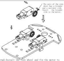
Setp2:Install the code wheel and fix the motor to the chassis. (Attention, the copper sheet of the leading wire of the motor should face outward, the same side of the wheel)
