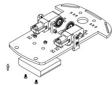
Setp4:Insert the screws and fix the battery container.
