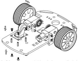
Setp5:Insert the spacer and tighten the 8 screws to fix the hammer caster. Hold tight and insert the motor(protecion fastener) to the wheel.Installation completed.
