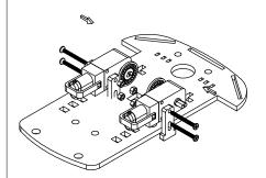
${\tt Setp3:} Fix$  the motor to the chassis, then insert and tighten the screws.
