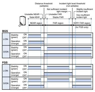
Note: 1 . If the stability indicator is lit, the detection/no detection status is stable
