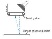
If the sensing object has a glossy surface, however, incline the Sensor by 5° to 10° as shown in the illustration, provided that the Sensor is not influenced by background objects.
