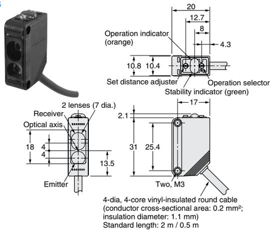
4-dia, 4-core vinyl-insulated round cable (conductor cross-sectional area: 0.2 mm<sup>2</sup>; insulation diameter: 1.1 mm) Standard length: 2 m / 0.5 m
