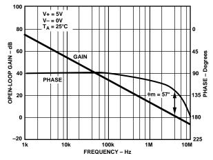
TPC 10. Open-Loop Gain, Phase vs. Frequency @ 5 V
