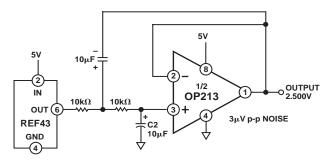
Figure 7. Low Noise Voltage Reference
