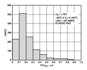
TPC 2c. OP413 Temperature Drift (TCV<sub>os</sub>) Distribution @  $\pm$ 15 V
