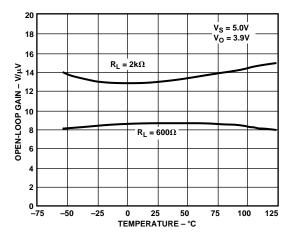
TPC 8. Open-Loop Gain vs. Temperature @ 5 V
