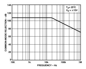
TPC 20. Common-Mode Rejection vs. Frequency @ $\pm$ 15 V
