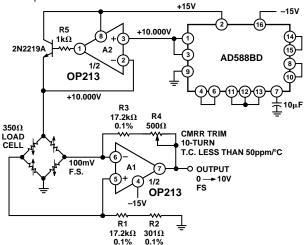
Figure 1. Precision Load Cell Scale Amplifier
