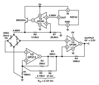
Figure 2. Single Supply Strain-Gage Amplifier
