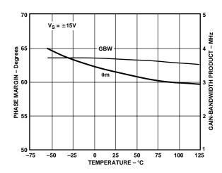
TPC 18. Gain Bandwidth Product and Phase Margin vs. Temperature @  $\pm 15~V$
