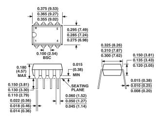
COMPLIANT TO JEDEC STANDARDS MO-095AA CONTROLLING DIMENSIONS ARE IN INCHES; MILLIMETERS DIMENSIONS (IN PARENTHESES)
