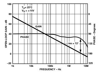
TPC 13. Open-Loop Gain, Phase vs. Frequency @ ±15 V
