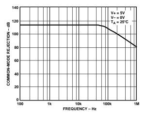
TPC 17. Common-Mode Rejection vs. Frequency @ 5 V
