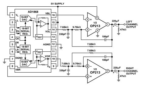
Figure 8. 5 V Only 18-Bit Stereo DAC
