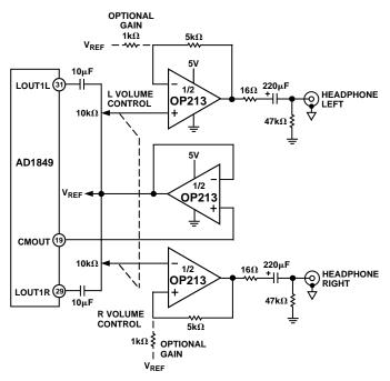
Figure 9. Headphone Output Amplifier for Multimedia Sound Codec
