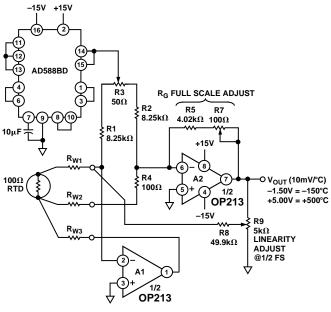
Figure 3. Ultraprecision RTD Amplifier
