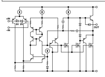
Figure 12. OP213 Simplified Schematic
