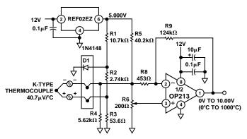
Figure 4. Accurate K-Type Thermocouple Amplifier
