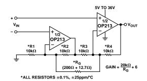
Figure 5. Ultralow Noise, Single Supply Instrumentation Amplifier
