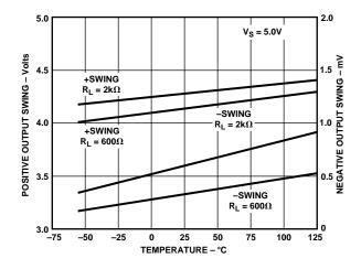
TPC 4. Output Swing vs. Temperature and R<sub>L</sub> @ 5 V
