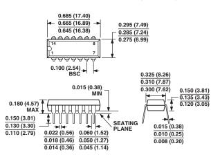
COMPLIANT TO JEDEC STANDARDS MO-095-AB CONTROLLING DIMENSIONS ARE IN INCH; MILLIMETERS DIMENSIONS (IN PARENTHESES) ARE ROUNDED-OFF MILLIMETER EQUIVALENTS FOR REFERENCE ONLY AND ARE NOT APPROPRIATE FOR USE IN DESIGN
