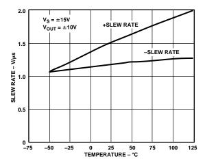
TPC 30. Slew Rate vs. Temperature @  $\pm 15$  V (-10 V  $\leq V_{OUT} \leq \pm 10.0$  V)
