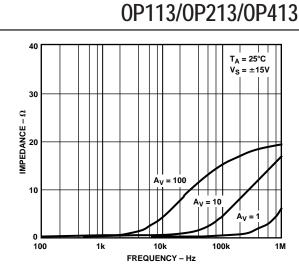
TPC 24. Closed-Loop Output Impedance vs. Frequency @  $\pm 15~V$
