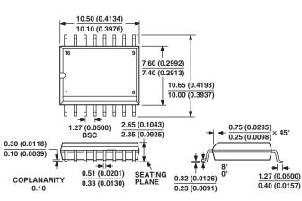
COMPLIANT TO JEDEC STANDARDS MS-013AA CONTROLLING DIMENSIONS ARE IN MILLIMETERS; INCH DIMENSIONS (IN PARENTHESES) ARE ROUNDED-OFF MILLIMETER EQUIVALENTS FOR REFERENCE ONLY AND ARE NOT APPROPRIATE FOR USE IN DESIGN
