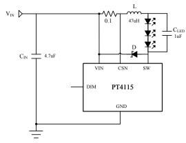
A value of 1uF will reduce the supply ripple current by a factor three (approx.). Proportionally lower ripple can be achieved with higher capacitor values. Note that the capacitor will not affect operating frequency or efficiency, but it will increase start-up delay and reduce the frequency of dimming, by reducing the rate of rise of LED voltage.
