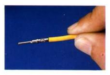
1 Grasp crimped contact approximately (25.4 mm) one inch behind the contact barrel.
