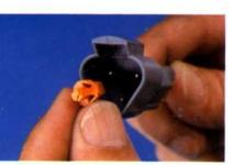
4 Once all contacts are in place, insert orange wedge with arrow pointing toward exterior locking mechanism. The orange wedge will snap into place. Rectangular wedges are not oriented. They may go in either way.
