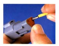
3 Hold the rear seal in place, as removing the contact will displace the seal.
