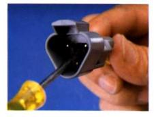
2 To remove the contacts, gently pull wire backwards, while at the same time releasing the locking finger by moving it away from the contact with a screwdriver.
