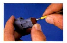
3 Push contact straight into connector grommet until a click is felt. A slight tug will confirm that it is properly locked in place.
